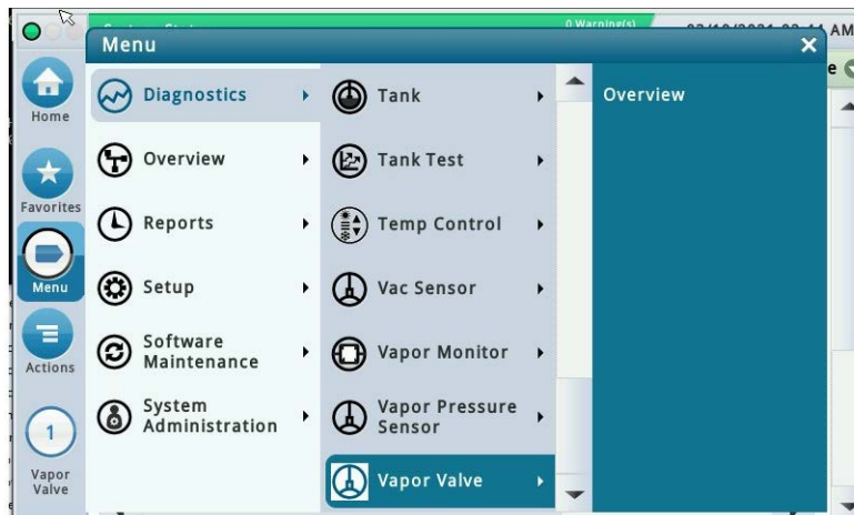
Figure 35. Example Vapor Valve Diagnostic Overview Screen
