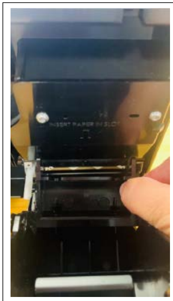
Figure 5-36: Disengaging the Printer Platen
