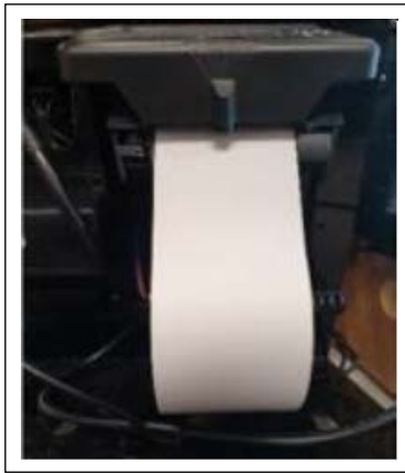
Figure 5-6: Correct Paper Loaded Position
