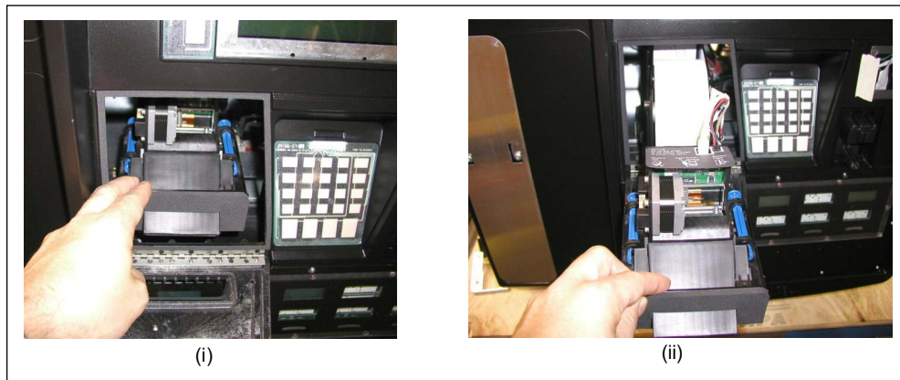
Figure 5-28: Opening Door and Pulling out Slide
