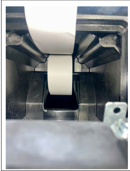
Figure 5-2: Roll and Spindle in the Printer Channel
