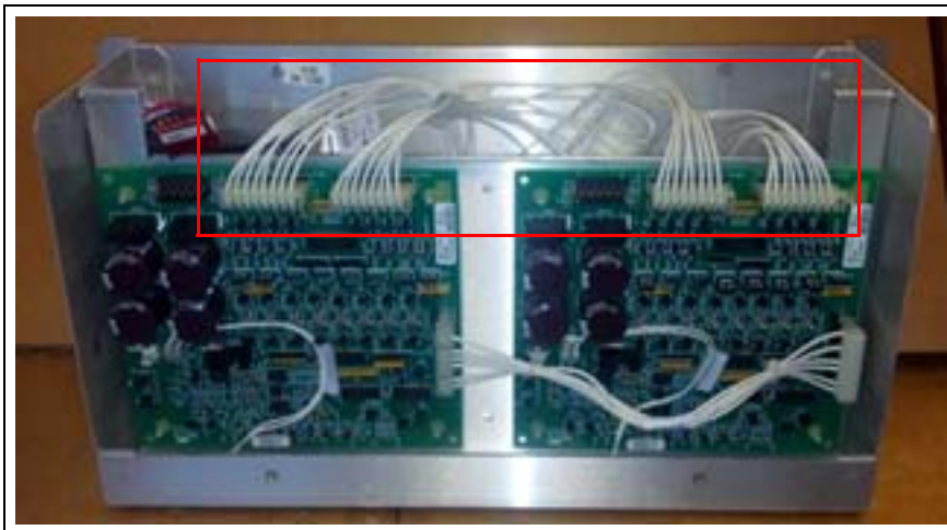
Figure 15: Removing Field Wiring Connectors
