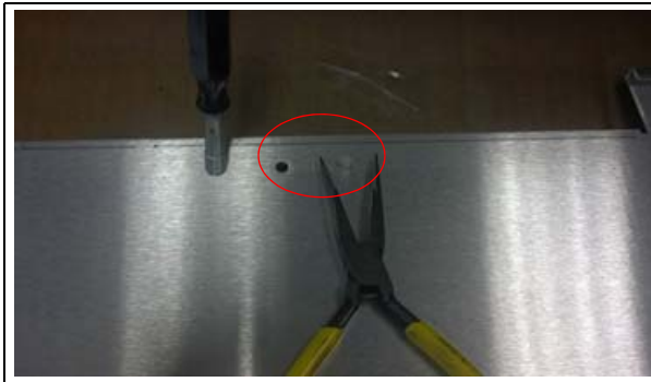
Figure 16: Squeezing Retaining Clips to Remove Standoff
