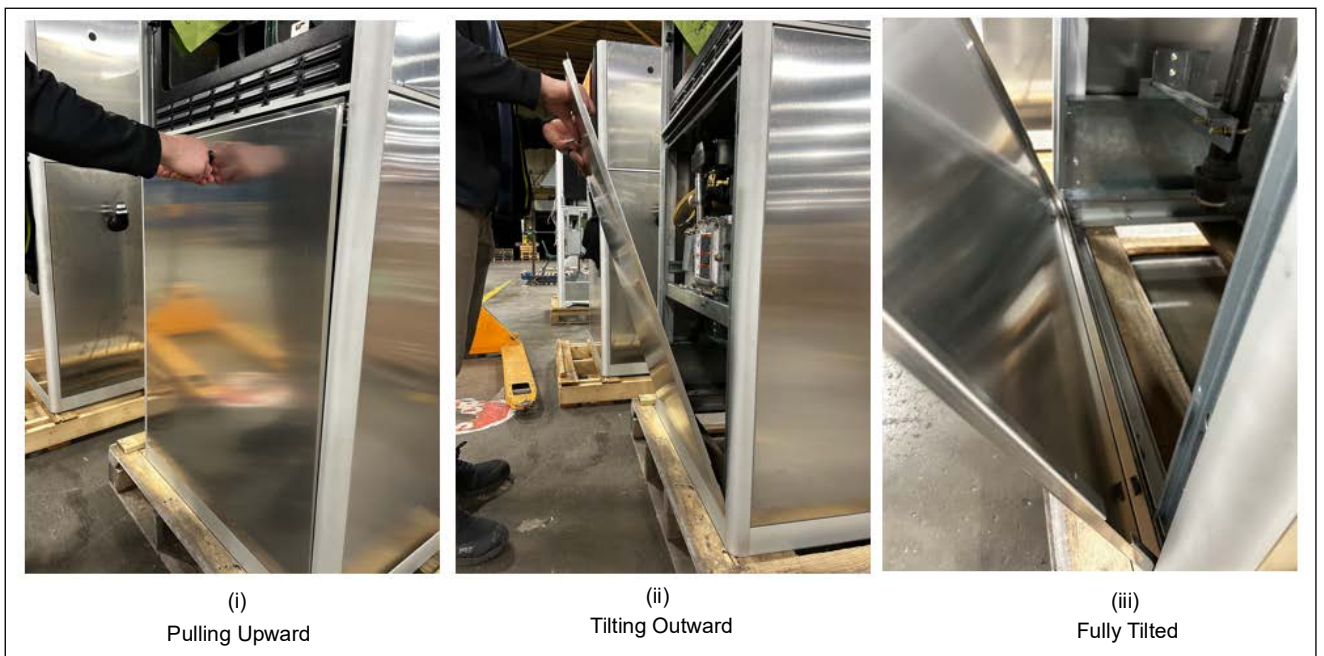
Figure 4-8: Opening the Lower Panel Door
