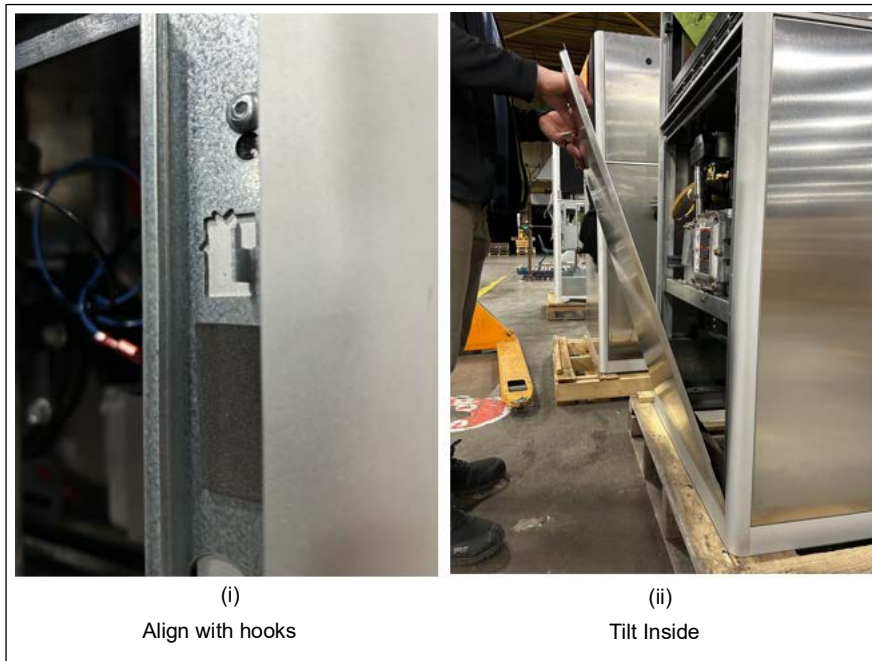
Figure 4-11: Closing the Lower Panel Door
