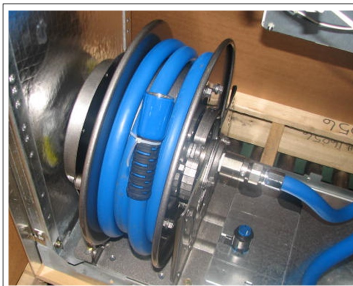
Figure 6-46: Securing the End of the Hose
