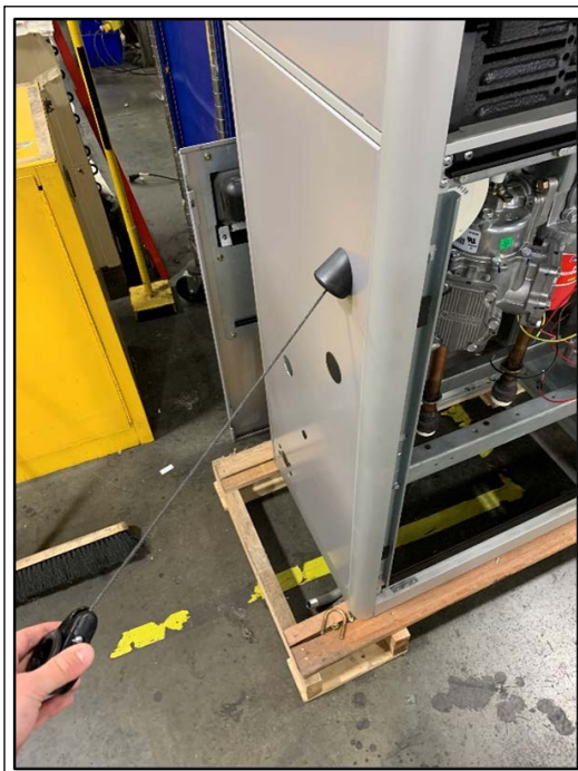
Figure 6-26: Adjusting the Reel Tension
