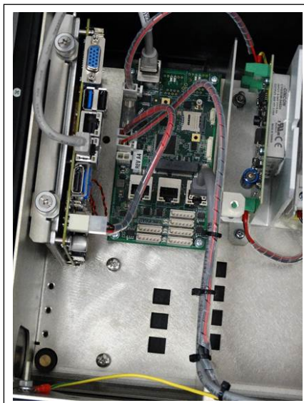
Figure 5-47: Connected to CommBoard
