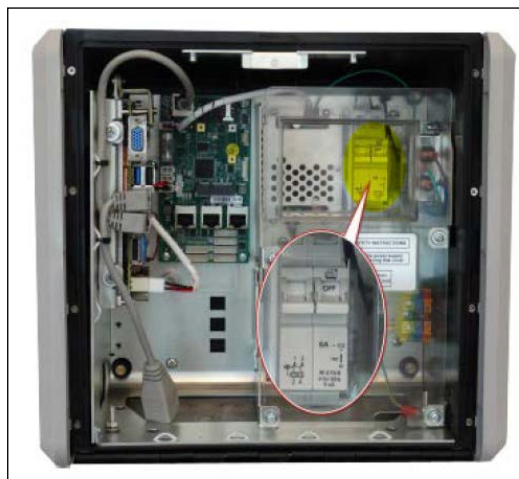
Figure 5-39: Main Power Switch - OFF
