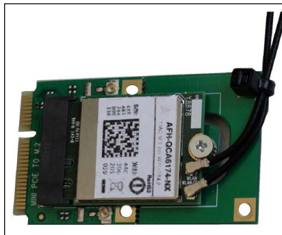
Figure 5-29: Antennas Fastened With Cable Tie
