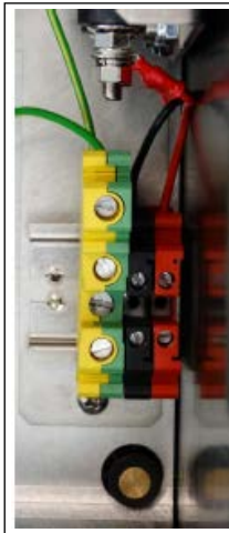
Figure 5-17: DC Power Supply Connected to GND/Neutral/Line
