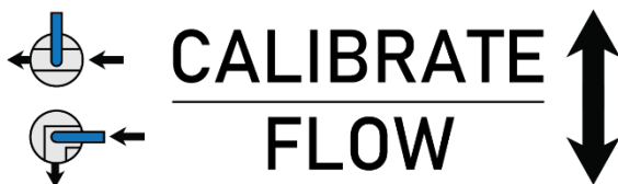
Figure 24: 3-Way Handle Position for Biofuel
