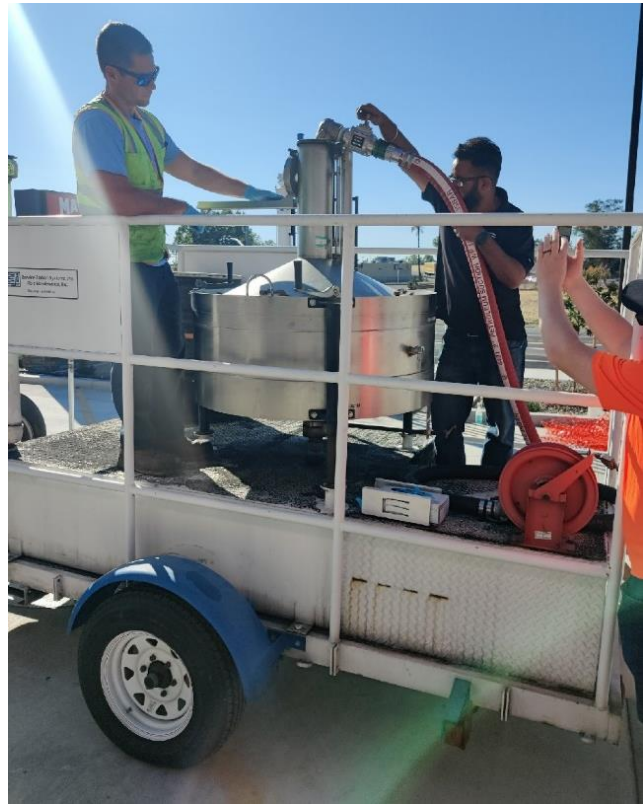
Figure 25: Calibration using a 100 Gal Volumetric Prover
